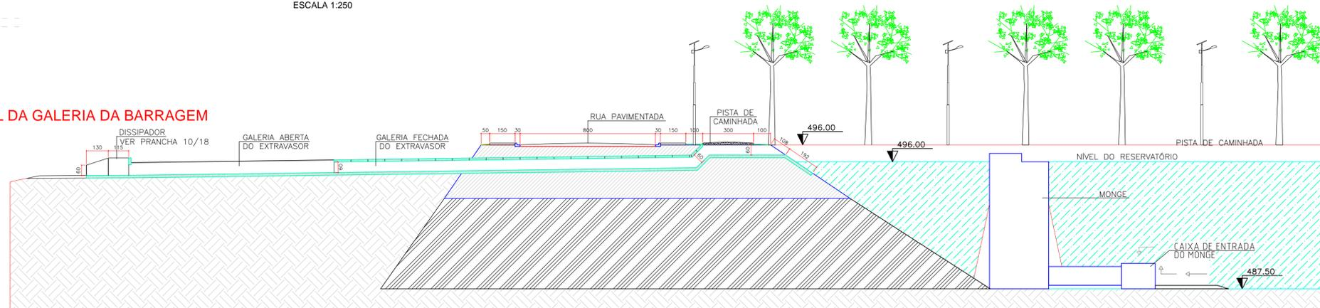
DETALHE 01 - CORTE AA - EXTRAVASOR DA BARRAGEM
